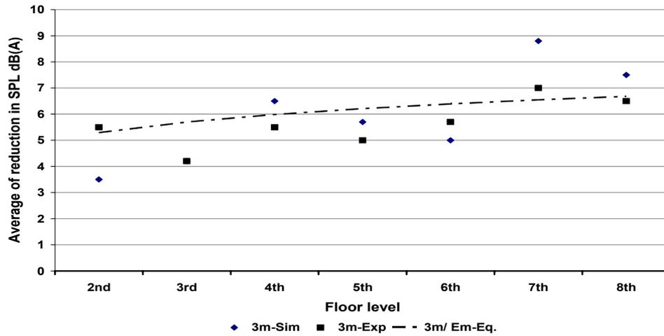
Fig. 14. Reduction Average for a 3m-balcony depth, ◆ simulation results, ■ measurements results, and --- empirical equation results.
