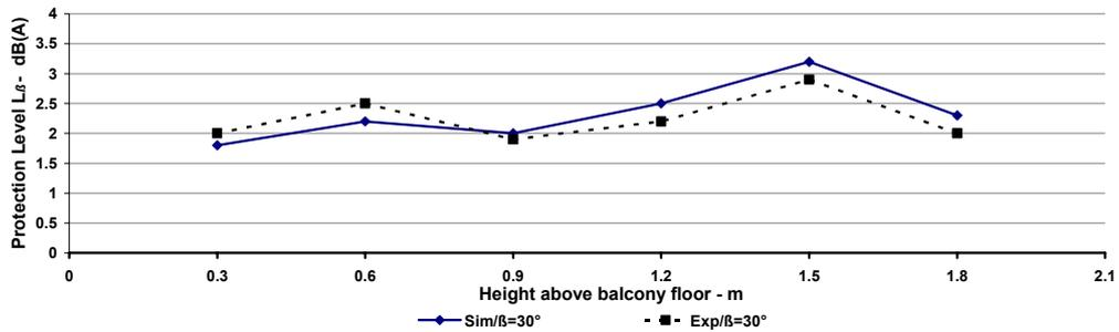
Fig. 20. Protection level provided by an inclined parapet ( $\beta = 30^\circ$ ) for a balcony with 2m and at the centre of its back wall (7<sup>th</sup> floor),  $\blacklozenge$  straight line represents the simulation results,  $\blacksquare$  dashed line represents the measurements results.
