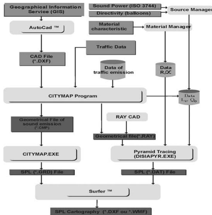
Fig. 4 Schematic representation of the pyramid tracing model (DISIAPYR<sup>®</sup>) [2].
