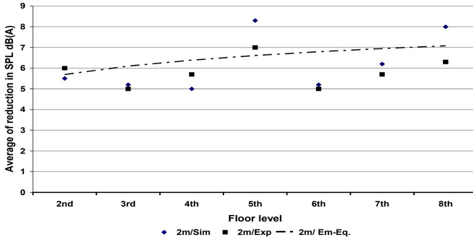
Fig. 12. Average reduction for a 2m-balcony depth, ◆ simulation results, ■ measurements results, and - - - empirical equation results.
