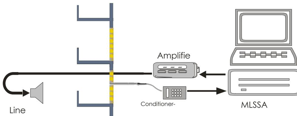
Fig. 8. Schematic representation of measurement system.
