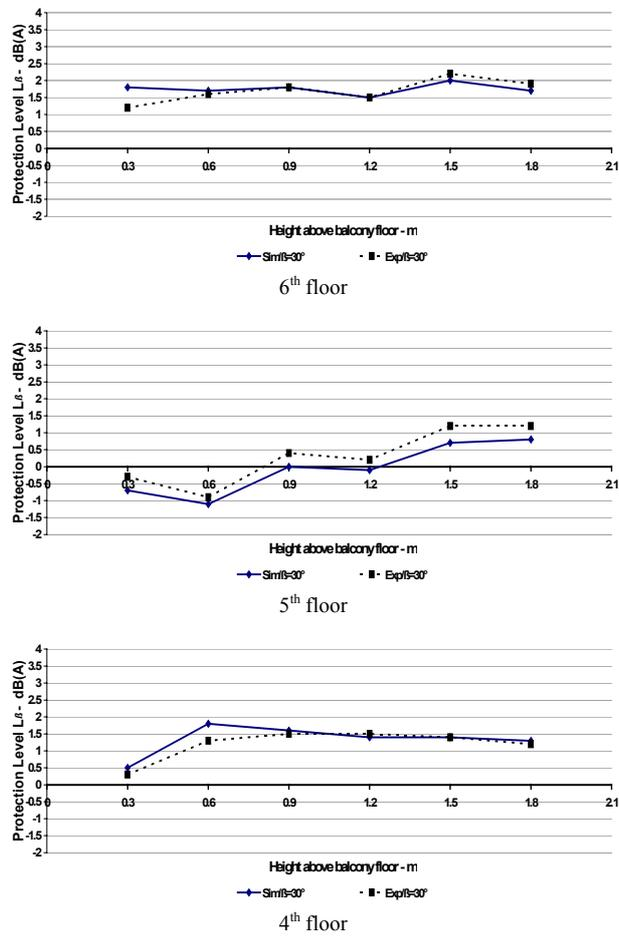
Fig. 19. Floors and ceiling reflection effects at the 4<sup>th</sup>, 5<sup>th</sup>, and 6<sup>th</sup> floors for a 2m-balcony depth with inclined parapet ( $\beta = 30^\circ$ ).
