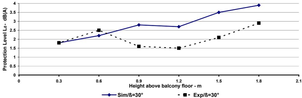
Fig. 22. Protection level provided by an inclined parapet ( $\beta = 30^\circ$ ) for a balcony with 3m and at the centre of its back wall (3<sup>rd</sup> floor),  $\blacklozenge$  straight line represents the simulation results,  $\blacksquare$  dashed line represents the measurements results.
