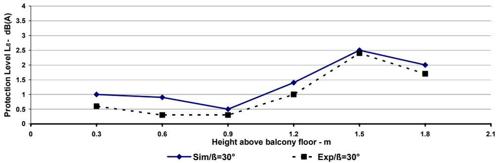
Fig. 17. Protection level provided by an inclined parapet ( $\beta = 30^\circ$ ) for a balcony with 1m and at the centre of its back wall (8<sup>th</sup> floor),  $\blacklozenge$  straight line represents the simulation results,  $\blacksquare$  dashed line represents the measurements results.
