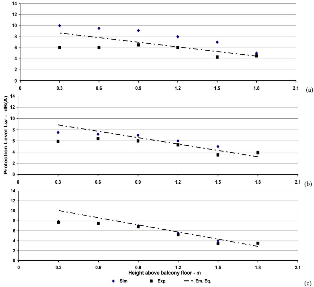
Fig. 13. Protection level for a 2m-balcony depth at the centre of its back wall,  $\blacklozenge$  simulation results,  $\blacksquare$  measurements results, and - - empirical equation results for the (a) 8<sup>th</sup>, (b) 6<sup>th</sup>, and (c) 4<sup>th</sup> floors.
