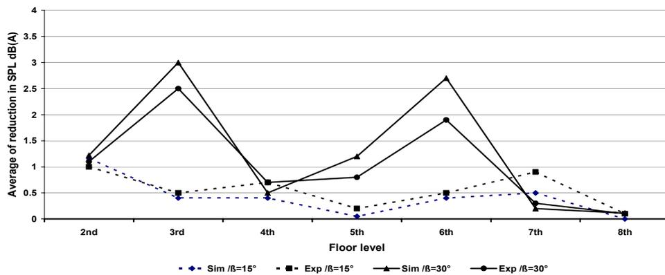
Fig. 21. Reduction average provided by inclined parapets ( $\beta = 15^\circ$  and  $30^\circ$ ) for a 3m balcony 3m depth, (Sim) simulation results, and (Exp) measurements results.
