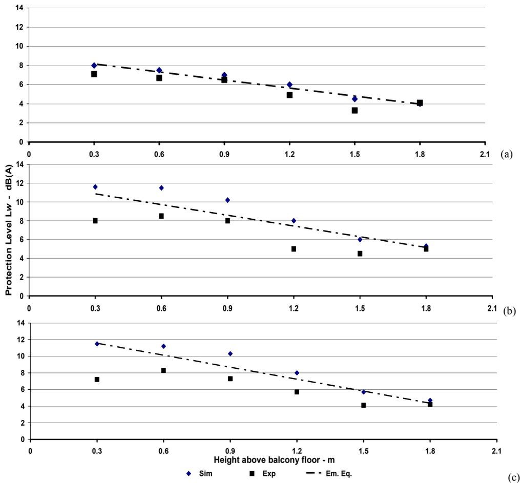
Fig. 11. Protection level for a 1m-balcony depth at the centre of its back wall,  $\blacklozenge$  simulation results,  $\blacksquare$  measurements results, and  $- \cdot -$  empirical equation results for the (a) 8<sup>th</sup>, (b) 6<sup>th</sup>, and (c) 4<sup>th</sup> floors.
