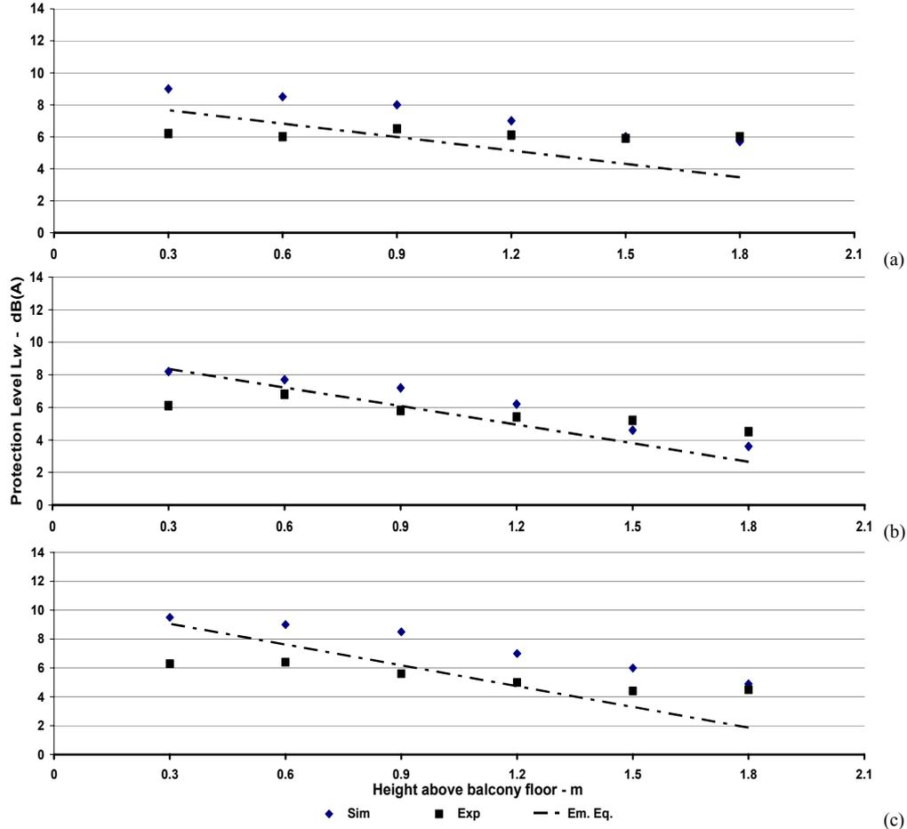
Fig. 15. Protection level for a 3m-balcony depth at the centre of its back wall,  $\blacklozenge$  simulation results,  $\blacksquare$  measurements results, and  $- -$  empirical equation results for the (a) 8<sup>th</sup>, (b) 6<sup>th</sup>, and (c) 4<sup>th</sup> floors.
