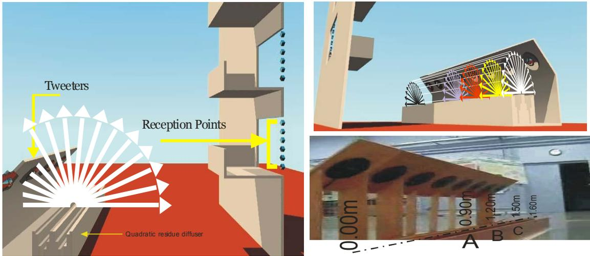
Fig. 6. Line source with a quadratic residue diffuser.
