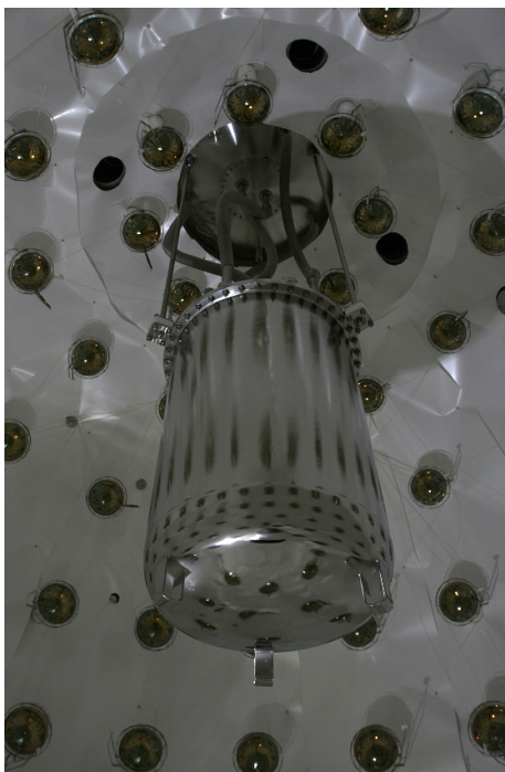
Figure 2. The Liquid Scintillator Veto (LSV). The picture shows the cryostat of the DarkSide-50 LAr TPC hanging from the top.
