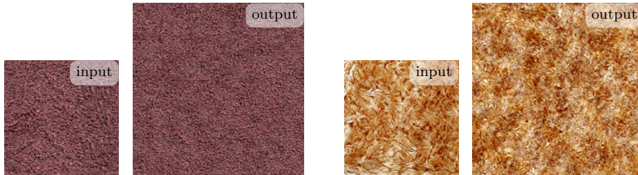
Figure 3: Synthesis results of the Heeger and Bergen method [33]. This method works for microtextures. For more structured texture images it fails. Two examples are shown: a successful synthesis on the left and a failure case on the right.
