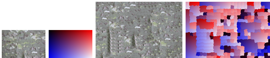
Figure 12: From left to right: texture sample, position map, synthesized image and synthesis map. The synthesis map shows for each synthesized patch its initial position in the texture sample. It allows then to identify exactly the verbatim copy regions (they correspond to continuous color areas of the map) and the repetitions (corresponding to repeated continuous patches of the same color).
