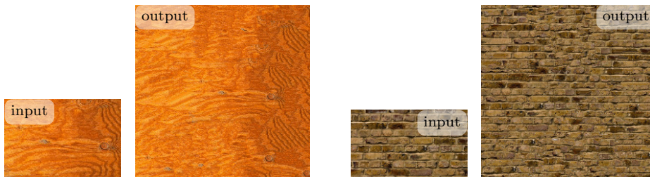
Figure 8: Synthesis results of the Efros and Leung method [13]. Left: the example shows the garbage growing effect. Right: the example shows the strength of this method to synthesize macrotextures. The patch size used for both synthesis is n = 40 .
