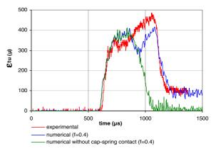
**Fig. 13.** Numerical and experimental evolutions of the circumferential strain on the tube (at the position of the gauge).
