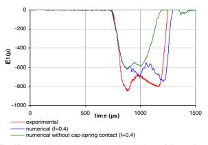
**Fig. 12.** Numerical and experimental evolutions of the strain of the output bar (at the position of the gauge).
