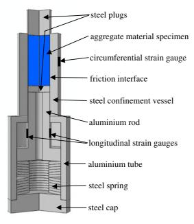
Fig. 1. Sketch of the confined friction set-up.
