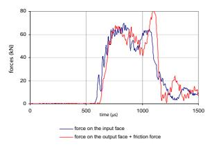
**Fig. 15.** Numerical evolution of the forces applied on the specimen. "Input face" denotes the specimen face on the input bar side and "output face" denotes the specimen face on the output bar side.
