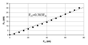
Fig. 2. Experimental evolutions of  $F_m$  and  $F_{ro}$  respectively the force applied by the machine and the normal force in the rod.
