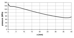
Fig. 6. Contact pressure along the interface at the maximum load. The position z = 0 corresponds to the top of the specimen (figure 1).
