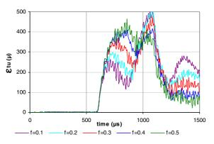
**Fig. 10.** Numerical evolution of the circumferential strain on the tube (at the position of the gauge), depending on *f* magnitude.
