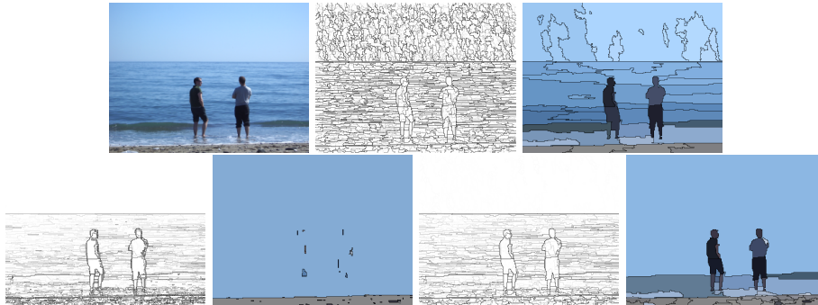
Fig. 1. First row from left to right: original image, saliency map and the 50 th highest level set of area based hierarchy. Second row from left to right: saliency map and the 50 th highest level sets of dynamics and the combination of area and dynamics based hierarchies.
