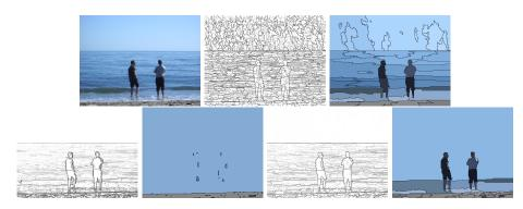
**Fig. 1.** First row from left to right: original image, saliency map and the  $50^{th}$  highest level set of area based hierarchy. Second row from left to right: saliency map and the  $50^{th}$  highest level sets of dynamics and the combination of area and dynamics based hierarchies.
