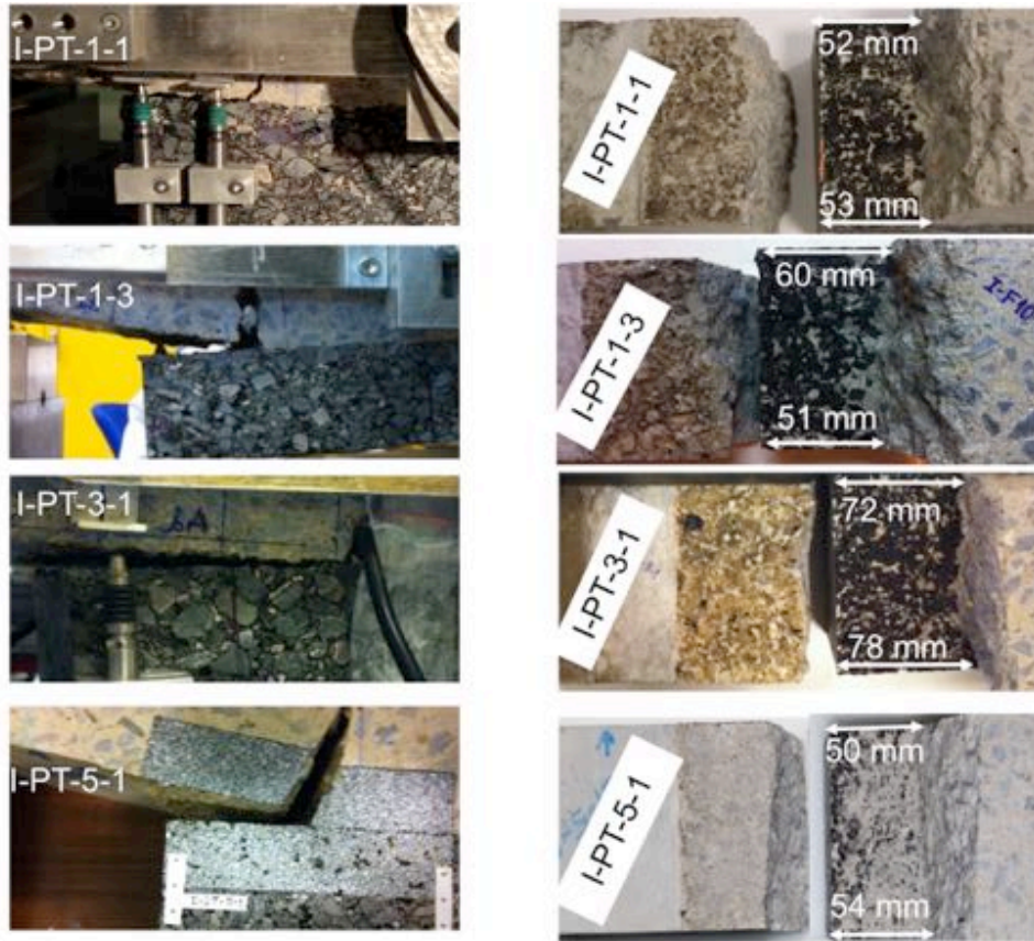
Figure 7. Visual debonding fracture aspect (lateral and top views) of the 4 specimens tested in dry condition
