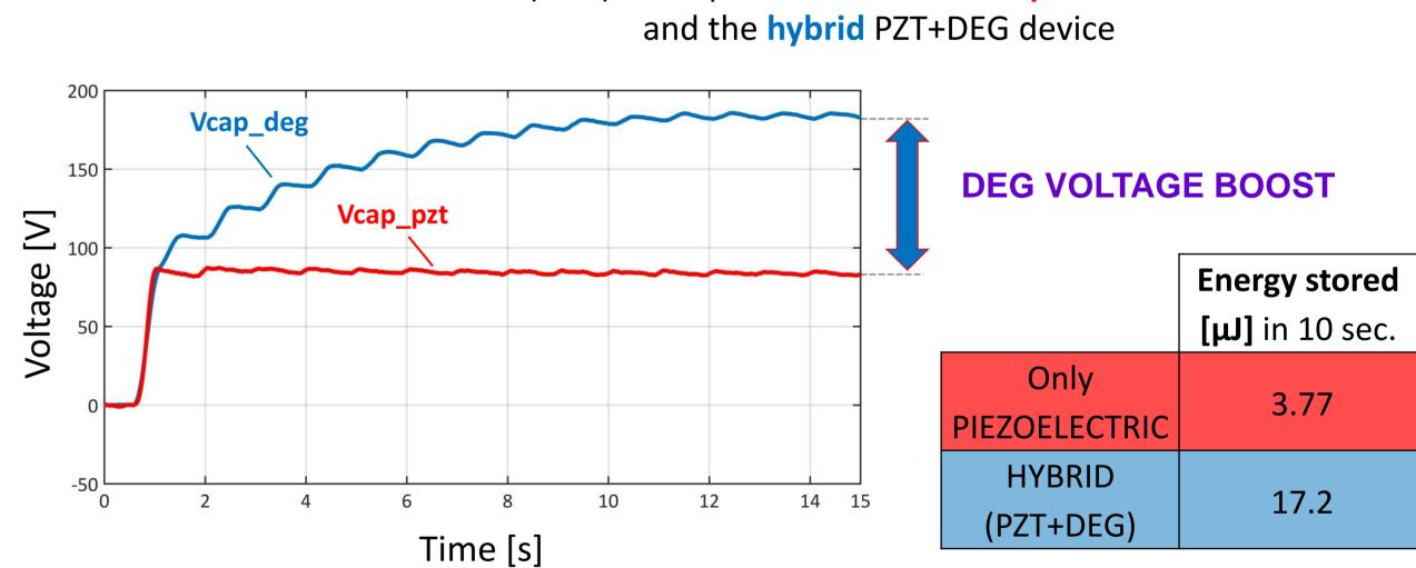
This value of energy represents the <u>FINAL useful energy</u> at the end of the energy harvesting cycle (Energy transduction + Power management unit)
