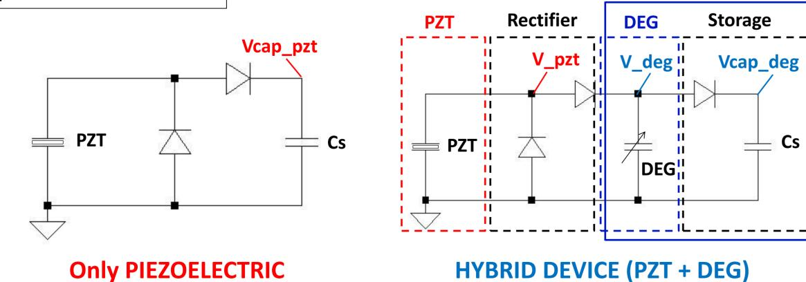
The voltage output generated by the compression force on the piezoelectric material is further boosted by the DEG energy cycle, thus increasing the harvested energy output
