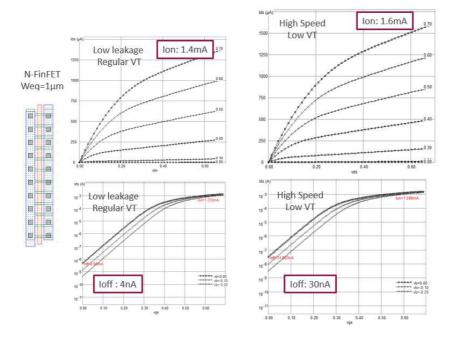
Figure 13: Id/Vd characteristics of the low leakage and high speed n-channel FinFET devices.
