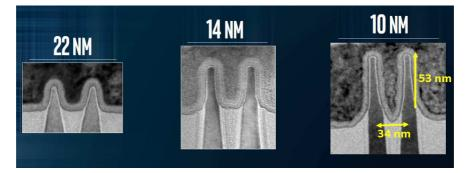
Figure 8: FinFet technology from Intel [Mistry2017] with increased fin height to improve the
