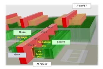
Figure 10: 3D view of the FinFET and illustrations of the Fin height (HF), Fin Thickness (TF) and Fin Length (LG).
