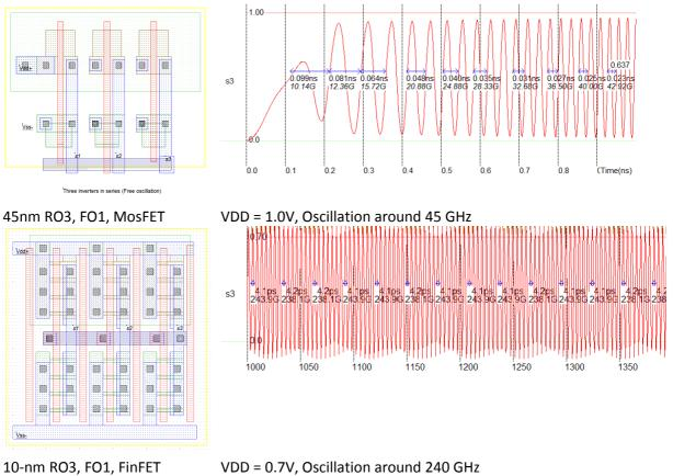
Figure 19: Considerable speed improvement is observed between 45-nm 3-stage ring oscillator based on MosFET and 10-nm 3-stage ring oscillator based on FinFET
