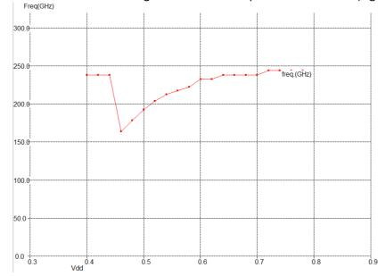
Figure 21: Modify VDD to extract the minimum operating voltage of the ring oscillator.
