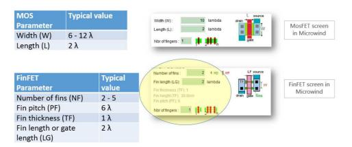
Figure 9: The introduction of the FinFET in Microwind, and comparison with traditional MosFET
