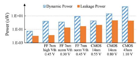
Figure 1: The reduction of feature sizes from 45 to 7nm may induce drastic gains in power consumption and leakage power [Xie2015]
