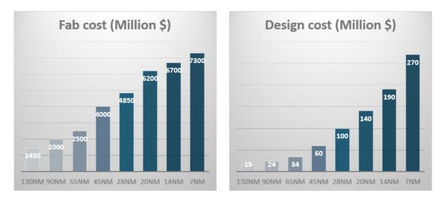
Figure 4: The extraordinary increase of the fab cost: more than 7 billion \$ for a 10-7-nm process, and associated chip design cost as high as 270M\$ for a run in 7-nm.
