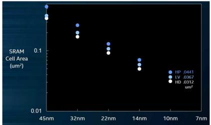
Figure 23: Reduction of the 6T-SRAM memory from 45-nm to 10-nm process of Intel, reaching 0.03µm2 for the most compact design [Miustry2017]
