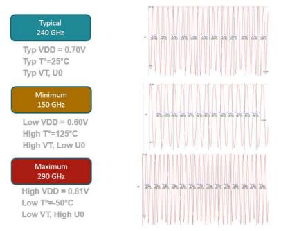
Figure 22: Typ/Min/Max simulation using PVT analysis
