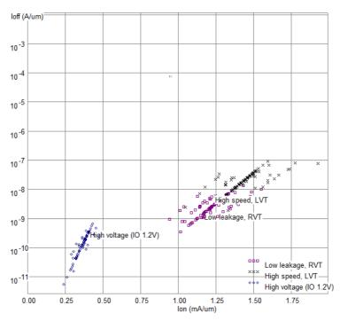
Figure 16: Ioff/Ion calculated on 100 samples of n-FinFET with random distribution of VT and U0, with a Gaussian distribution around the nominal value
