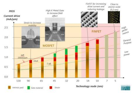
Figure 6: Increased switching speed capabilities over technology nodes
