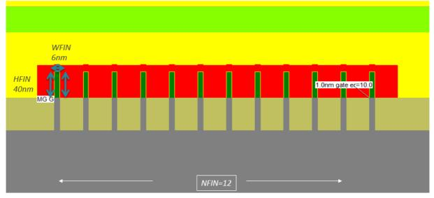
Figure 11: The equivalent width of a multi-fin FET
