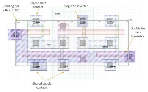
Figure 24: 6T-SRAM implementation in FinFET (SRAM-6T-10nm.MSK)
