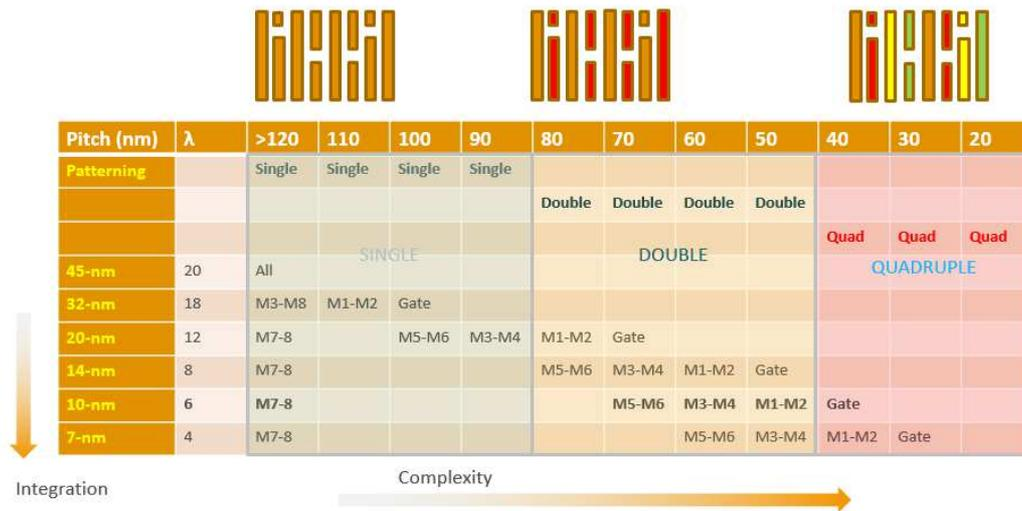
Figure 18: Single, double and quadruple patterning as a function of interconnect pitch [Brain2017]
