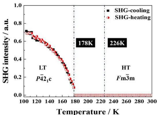
**Figure 3.** TR SHG curves obtained for the phase transition of 1 F A. Black square, upon cooling (1 K/min); red spot, upon heating (1 K/min). The signal appears/disappears at 178 K and increases with lowering the temperature down to 100 K.
