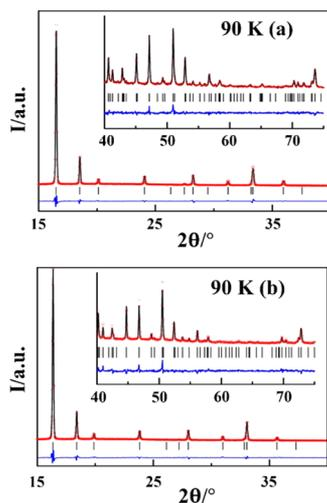
**Figure 4.** Experimental (red circles) and Rietveld refined (black line) diffraction patterns along with the difference profile (blue line) and Bragg reflections (vertical black sticks) of (a) the LT phase at 90 K and the (b) MT phase at 190 K. The insets show the high angle portion of each pattern (scaled to enhance their visibility).
