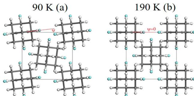
**Figure 5.** Crystal structure of 1 F A: (a) LT phase ( $P4_21c$ ,  $Z = 2$ ) at 90 K and (b) MT phase ( $P4_2/nmc$ ,  $Z = 2$ ) at 190 K. The fractional occupancy of 1/4 of the fluorine atoms (blue) remains unchanged across the MT ↔ LT transition.
