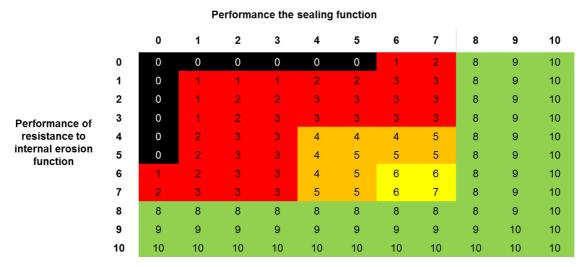
Figure 7. Truth table for combination the values of the performances of "sealing" and "resistance to internal erosion" functions.
