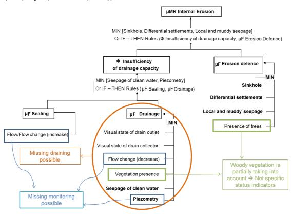
Figure 1. Hierarchical model for assessing an embankment dam built using homogenous fill equipped with a drain and monitoring instruments [ $\mu$  = performance;  $\Phi$  = phenomenon] (Curt, Peyras, & Boissier, 2010)
