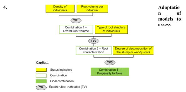
Figure 4. Structure of aggregation for assessing the propensity to flows linked to the presence of woody vegetation on the dam assessed.
