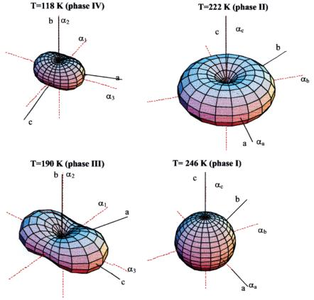
**Figure 6.** Three-dimensional thermal-expansion tensors of monoclinic phases IV and III at 118 and 190 K, respectively, and of the hexagonal phases II and I at 222 and 246 K, respectively, for  $c-C_5H_{10}O$  along its principal directions  $\alpha_1$ ,  $\alpha_2$ , and  $\alpha_3$  (dotted red line) together with the crystallographic axes a, b, and c (continuous back line). The full length of the  $\alpha_i$  axes corresponds to  $10^{-4}$  K<sup>-1</sup>.
