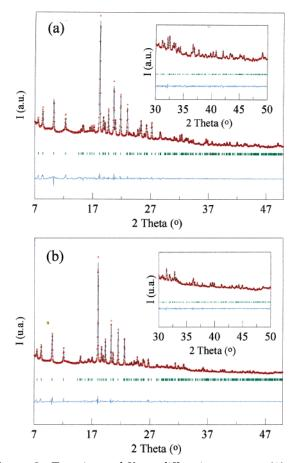
**Figure 2.** Experimental X-ray diffraction patterns ( $\bigcirc$ ) and simulated patterns using the FULLPROF program (-) of phases IV (a) and III (b) for c-C<sub>5</sub>H<sub>10</sub>O at 93 and 199 K along with the difference profile. (Inset corresponds to a five-times expanded vertical scale for the data from  $2\theta \geq 30^{\circ}$ ).
