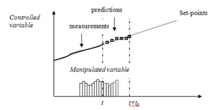
**Figure 1 : Predictive control principle**
