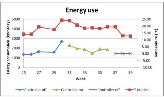
Figure 6 : Energy use related to refrigeration systems with controller on and off
