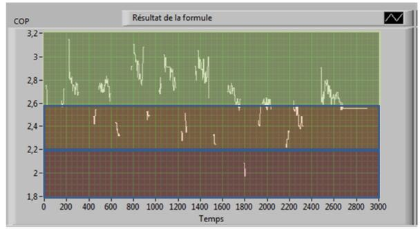
Figure 5 : Coefficient of performance with the controller activated
