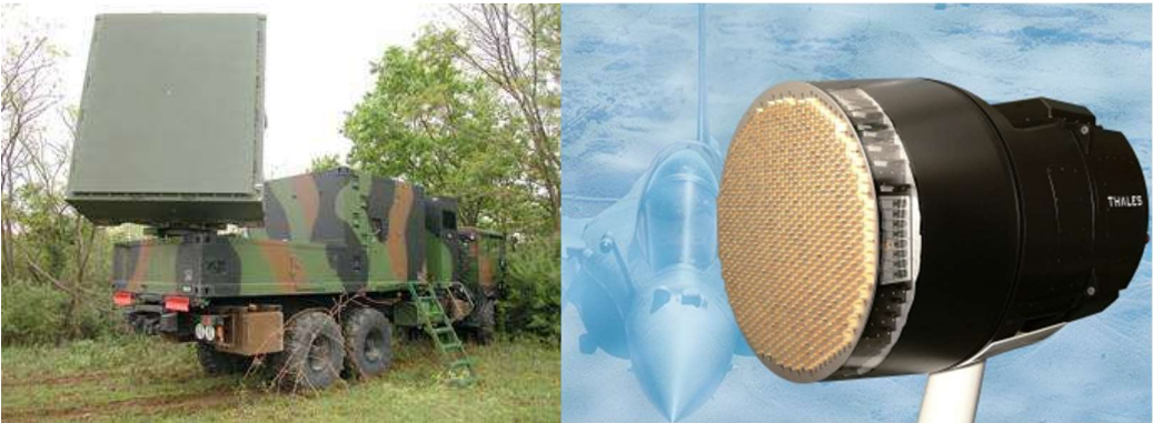
– Figure 7 : Modern radar active antennas (Courtesy of Thales): on the left, an active electronic scanning antenna (COBRA radar), and on the right an airborne fixed electronic scanning antenna (RBE2 radar of the Rafale) –
