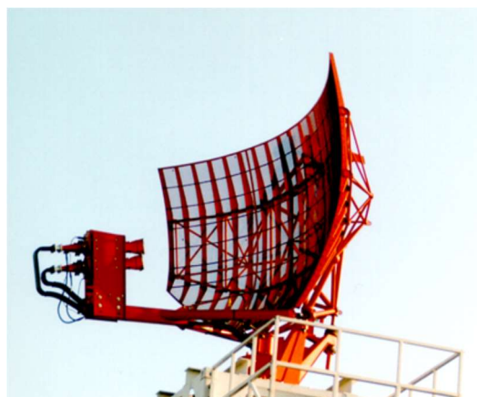
– Figure 4 : Rotating antenna with reflector, to monitor air traffic in the terminal area (range: 100 km) of an airport; We note the presence of 2 horns in the vicinity of the focus, to create 2 beams slightly offset in elevation –
