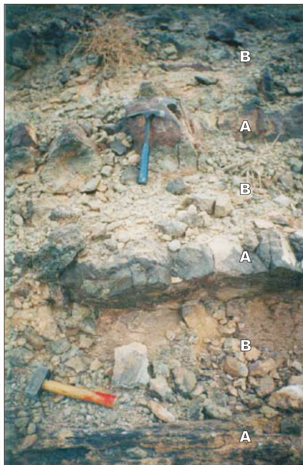
FIGURE 4. Example of volcanic flows (Unit B1, Djenien Bou-Rezg site). A) Massive aspect at the base. B) Vesicular upper part.
