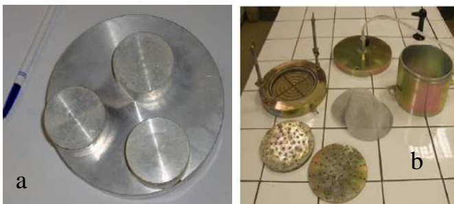
Figure 2: Kneading compaction tool (a) and permeameter (b).
