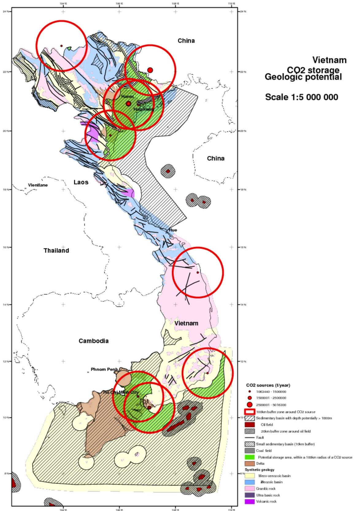
Figure 2: Geological formations potentially favorable for CO<sub>2</sub> storage in Vietnam (BRGM/TKV 2009, 34)
