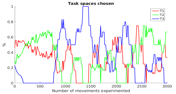
Fig. 8: Evolution of the choice of tasks of SGIM-ACTSCL: percentage of times each task is chosen across time
