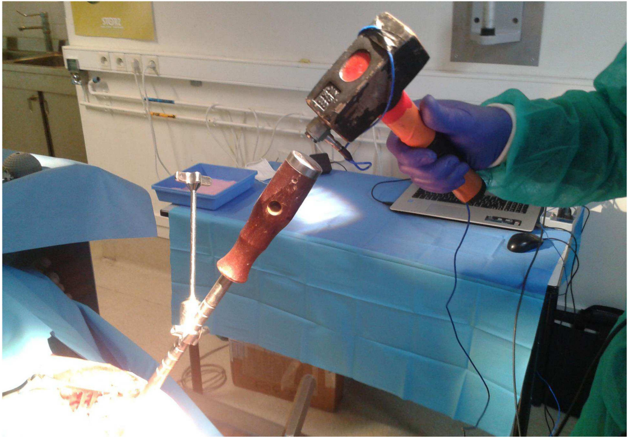
Fig 2. Illustration of the AC implant impact carried out with the measuring face of the impact hammer during the measurement protocol.
