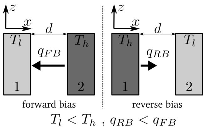
**Fig. 1** Two parallel planar bodies separated by a distance d. In forward bias configuration,  $T_1 = T_h$  and  $T_2 = T_c$ . In reverse bias configuration,  $T_1 = T_c$  and  $T_2 = T_h$ .
