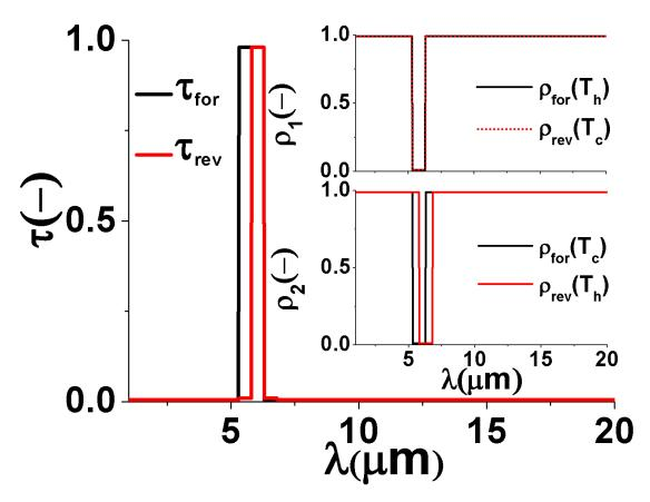
Fig. 2 The transmission coefficient in forward and reverse biased configurations and bodies 1 and 2 reflectivities in forward (top inset) and reverse bias (bottom inset) configurations. In both configurations,  $\lambda_{p,1}(T) = \lambda_W(T_h) = 5.8 \ \mu\text{m}$  while  $\lambda_{p,2}(T_c) = \lambda_{p,1}$  in forward bias and  $\lambda_{p,2}(T_h) = \lambda_{p,1} + \delta_{rev}\lambda_p$  in reverse bias where  $\delta_{rev}\lambda_p = \Delta\lambda/2$ .
