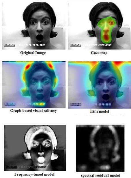
Fig. 5 Comparison of automatic detected salient regions with gaze map obtained from psycho-Visual experiment (see Section 3 for reference). First row: original image and average gaze map of fifteen observers. Second row: saliency maps obtained from GBVS [54] and Itti methods [53] (shown as heat maps). Third row: saliency maps obtained from FT [12] and SR methods [55].
