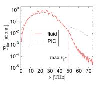
FIG. 6. Angularly integrated THz far field spectrum obtained from the fluid model (solid red line) and a PIC simulation (dashed gray line) in 3D. The red curve is the same as the one in Fig. 3(b) (iii) of the main article.
