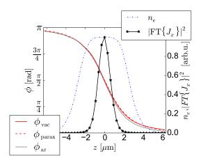
FIG. 10. Relative phase  $\phi(z)$  between the FH and SH field for laser and gas parameter same as in Fig. 7(a) on the optical axis (x = y = 0) as well as the electron density  $n_{\rm e}(z)$  (after the pulse has passed) and the on-axis peak power spectum of the THz current (< 60 THz). The electron density  $n_{\rm e}$  and the low frequency current source are normalized to one.
