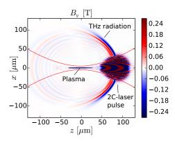
FIG. 1. Schematic illustration of two-color fs-laser-induced THz generation in a gas: A snapshot of the magnetic field  $B_y$  after the interaction of the laser pulse with the laser-induced plasma is presented. The two-color pulse and the generated THz radiation are indicated in the graph. The waist of the focused laser is tracked by the dark red lines, the position of the generated plasma is marked as a blue oval.
