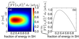
FIG. 13. Frequency integrated excitation source  $n_e \mathbf{E}$  for laser and gas parameter as in Fig. 7(a). In (a) the dependence on  $\phi$  and the fraction of energy in the SH pulse component is presented. In (b) a line-out of (a) for the optimal angle  $\phi = \pi/2$  is shown: The dependency on the SH pulse energy is not so critical. Already for few percent of the total energy in the SH field, the excitation source is reasonably strong.
