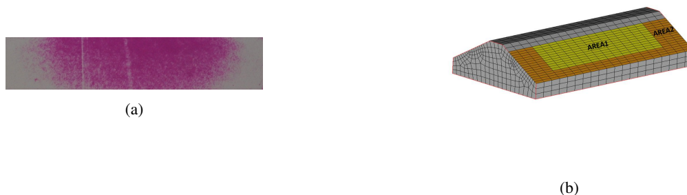
Figure 9: a) Pressure film print measured at the damper contact interface, b) FE model of the damper contact areas used for the pressure investigation.
