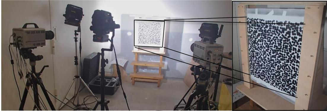
Figure 1. Stereo-correlation device comprising high speed camera and large scale target with coarse speckle pattern.
