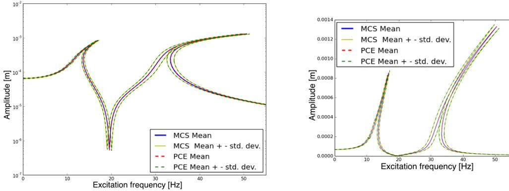
Figure 17: Mean and standard deviation responses for MCS and PCE, case D: Amplitude in logarithmic scale (left), Amplitude in linear scale (right).
