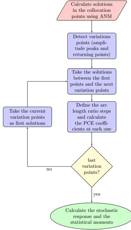
Figure 8: PCE + ANM with deterministic arc length ratio.
