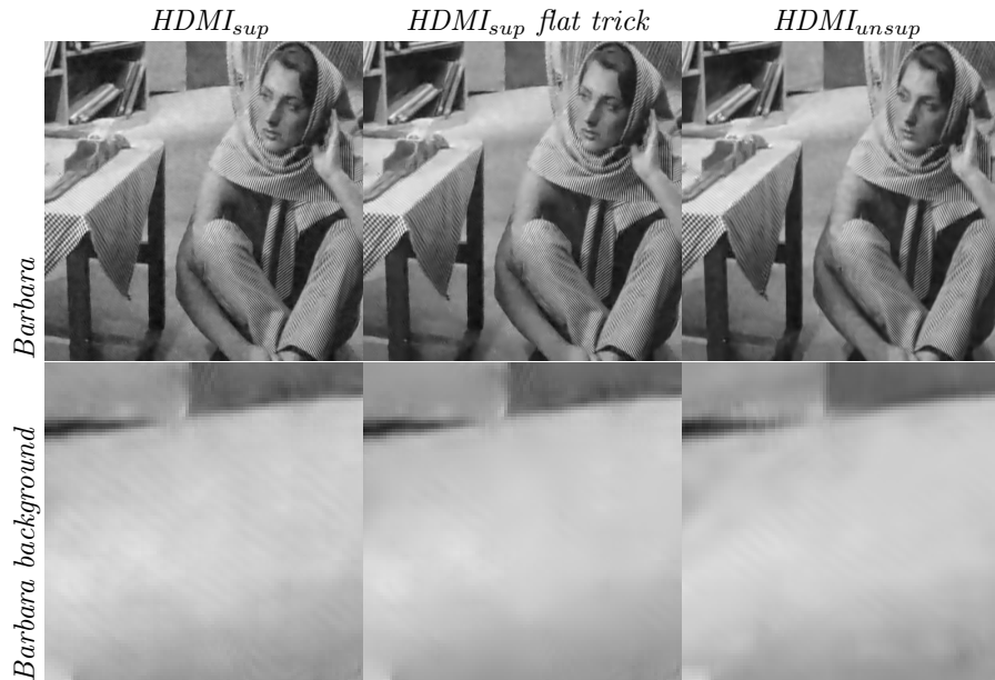
FIGURE 14. Result of HDMI denoising with K = 40 groups for the image Barbara with noise \sigma = 30 . Left HDMI (PSNR = 29.35dB), middle HDMI with the flat area trick (PSNR = 29.36dB), right unsupervised HDMI (PSNR = 29.11dB).
