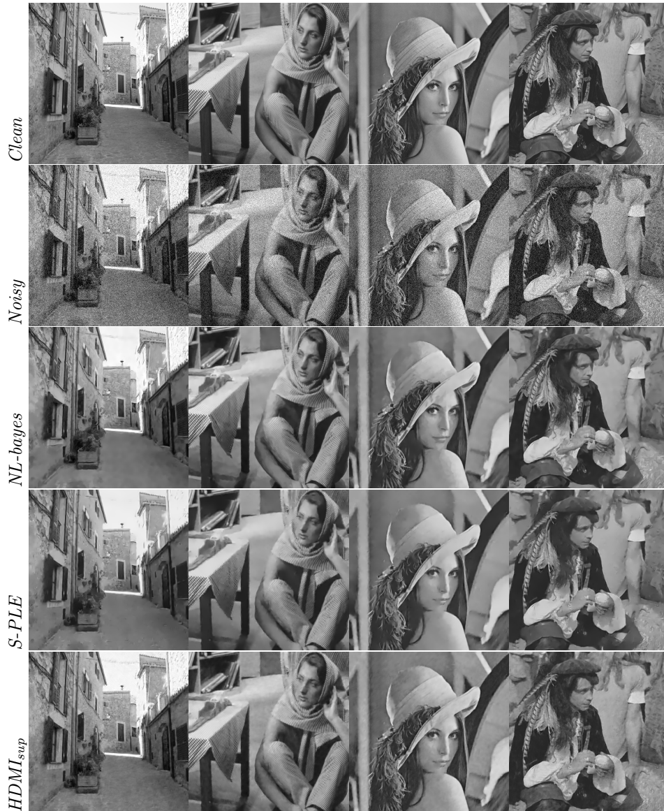
FIGURE 11. Comparative results on the grey-scale images Alley , Barbara , Lena and Man with \sigma = 30 . For each column, from top to bottom: original image, noisy image, NL-Bayes [25], SURE- PLE [36], HDMI. Images should be seen at full resolution on the electronic version of the paper.
