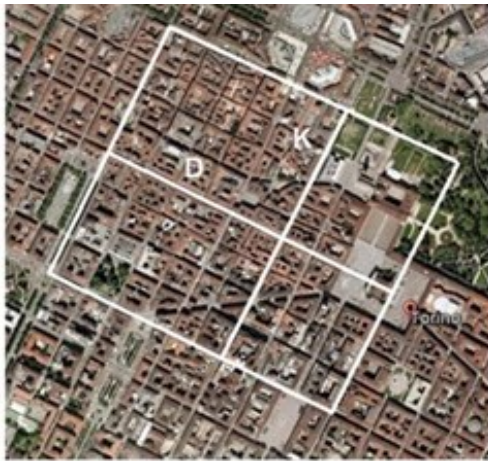
Figure 1: The Romans planned their towns with a precise regular scheme, based on two main streets, which crossed each other at right angles, at center of the settlement. These streets are the Decumanus (D) and the Kardo (K). A well-preserved example of the Roman town-planning is Torino: in this Google Earth image, we can easily see the rectangle of the Roman town, composed of several “insulae”, that is, of several square house-blocks.
