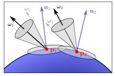
Figure 9: We merge two cache points that reproject onto the same pixel only if both their spatial and angular bandwidths overlap enough. In this example, while the two cache point's angular cones  $(\boldsymbol{\omega}_1, \boldsymbol{\omega}_2)$  align (gray), their spatial bandwidths at  $\boldsymbol{p}_1$  and  $\boldsymbol{p}_2$  do not overlap enough. Consequently, the two points will not be merged.
