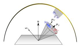
Figure 3: We only consider the frequency content of the (distant) incident lighting and visibility within the view-evaluated *BRDF footprint* (in yellow), defined as a cone centered about the mean reflection direction of the BRDF slice  $\mu_{\rho}$  with radius equal to three standard deviation  $\sigma_{\rho}$  of the BRDF lobe. Our visibility statistics, comprised of its mean  $\mu_{V}$  and three standard deviation  $\sigma_{V}$ , are also accumulated exclusively within this footprint.
