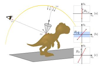
Figure 6: To estimate the screen-space bandwidth  $B_S$ , we start with the emitted (angular) bandwidth of the environment light  $B_{L_{\infty}}$  reduced to the BRDF's footprint (a), we then apply the BRDF bandlimit  $B_{\rho}$  (b) and modulated according to the curvature, foreshortening, and spatial transport (c). The angular bandwidth serves directly as the screen-space bandwidth estimate.
