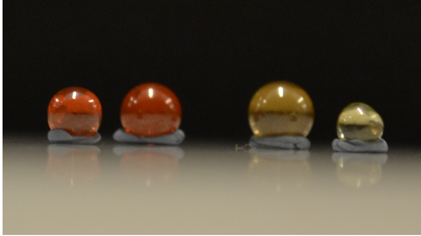
Fig. 1. Spin ice spherical crystals. From right to left Dy 2 Ti 2 O 7 sample A and sample B; Ho 2 Ti 2 O 7 sample C and sample D. Each sphere has a diameter ranging between 3 to 4 mm.
