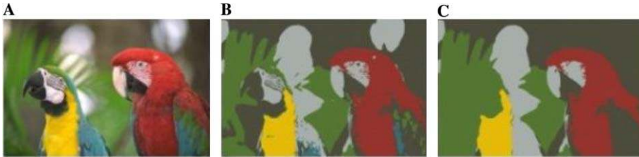
Fig. 6. The complete segmentation process. (A) Original image, (B) quantized image (10 classes, 2850 regions), and (C) segmented image (5 classes, 32 regions).
