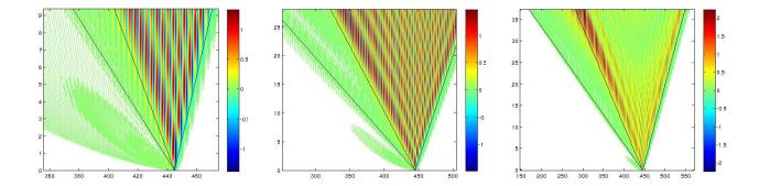
FIGURE 1. Three looks at the same time-evolution. The background wave has elliptic parameter m=0.5 hence period approximately 3.7081. Initial data for the perturbation  $W_0$  is the product of a sinus with a Gaussian. Dark lines start from the center of the Gaussian, and corresponds to linear group velocities.
