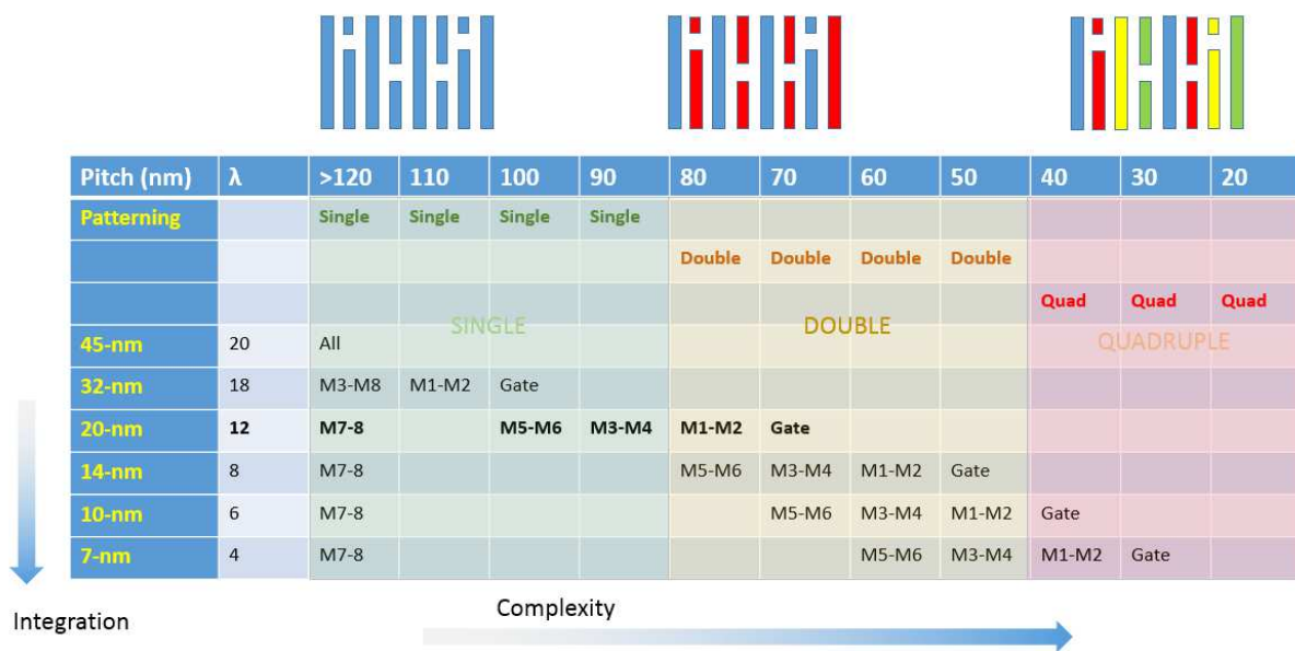
Figure 24: Single, double and quadruple patterning as a function of interconnect pitch [Brain2017]
