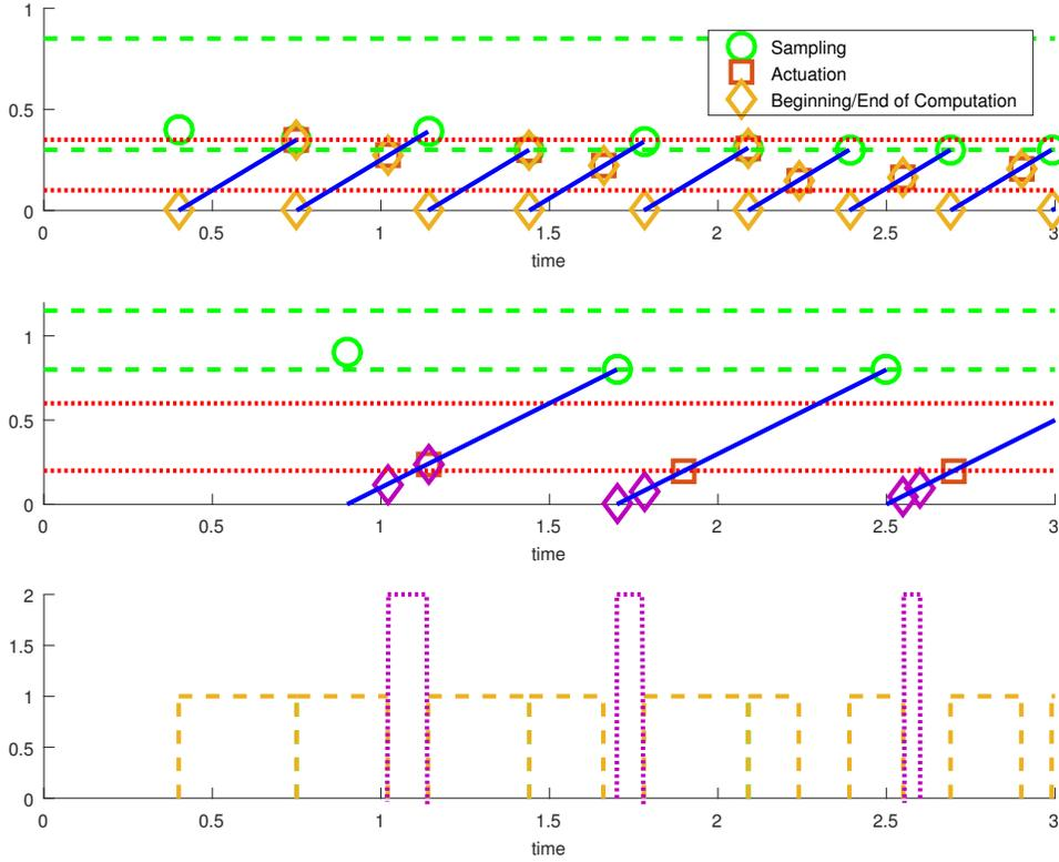
**Figure 2: Timing of events (sampling, beginning/end of computation, and actuation) for systems  $S_1$  (first plot) and  $S_2$  (second plot) during the first 3 seconds; dotted lines represent constraints on actuation instants, while dashed lines represent constraints on sampling instants. In the third plot, the dotted line represents  $\text{Com}(S_2, t)$  (less frequent) and the dashed line represents  $\text{Com}(S_1, t)$  (more frequent).**
