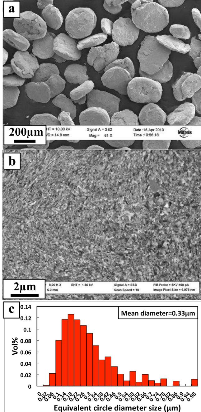
**Fig. 2. SEM image of (a) as-milled Fe14Cr powders showing an asymmetric particle's shape and (b) the nano-crystallites inside a particle powder observed from focused ion beam (FIB) cross-section. The histogram shown in (c) presents the crystallite size distribution.**
