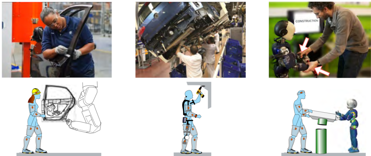
Figure 3: the three collaboration scenarios with the three different robot types: cobot or robotic manipulator, exoskeleton and humanoid robot.
