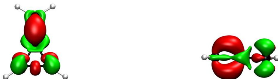
Figure 3: Top view (left) and side view of the electronic density difference map of MCP between the excited state ^1B_2 and the ground state ^1A_1 . An isovalue of + and -1.10^{-2} a.u. was used. Red contours correspond to areas where the electron density is smaller in the excited state than in the ground state.
