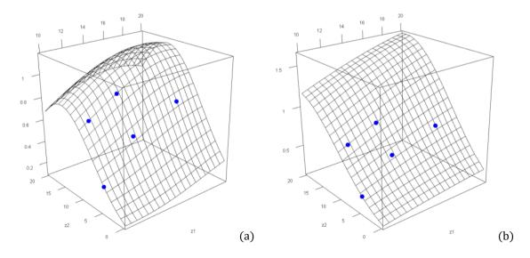
Fig. 2. (a) the usual kriging mean using the length parameter  $\hat{\theta}_{\text{CV}} = (9.05, 9.10)$  estimated by LOO criterion; (b) the function mode using the length parameters  $\hat{\theta}_{\text{CV}} = (25.17, 10.57)$  estimated by suited LOO criterion to inequality constraints.
