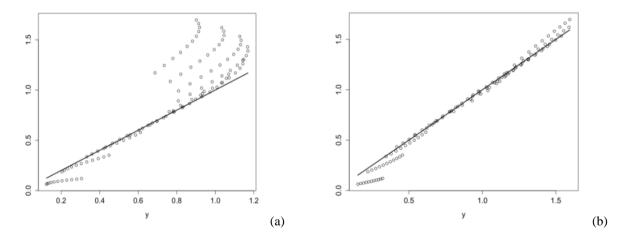
Fig. 3. the values estimated versus the real values using the usual kriging mean as an estimator (a) and mode (b).
