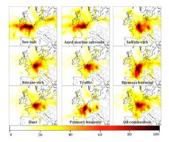
**Fig. 7.** Normalized PSCF values (in %) for all the identified sources in Lens.
