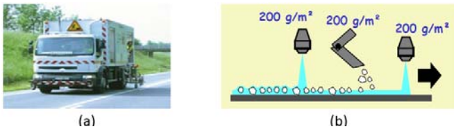
Figure 3. (a) A truck able to lay marking, (b) The "sandwich" lay technique.
