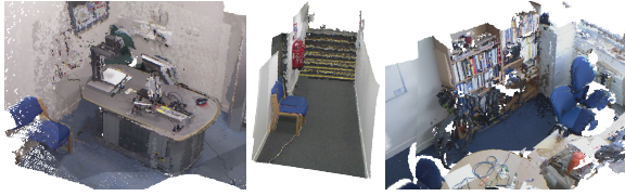
Figure 15: SUPER 4PCS based alignment of 5-6 scans for different scenes captured using Kinect.
