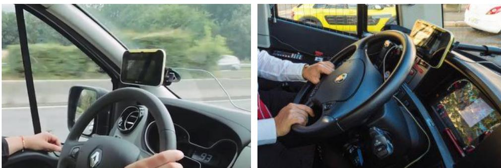
Figure 1 – Device's set up in a van (left) and in a bus (right)
