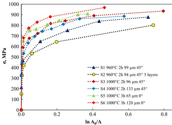
**Fig. 4.** True stress-strain curves of CP titanium samples tested in tomography. In the legend, the name of the sample is followed by diffusion bonding temperature and time, and by the void configuration parameters (intervoid spacing and angle of the voids with respect to the tensile axis).
