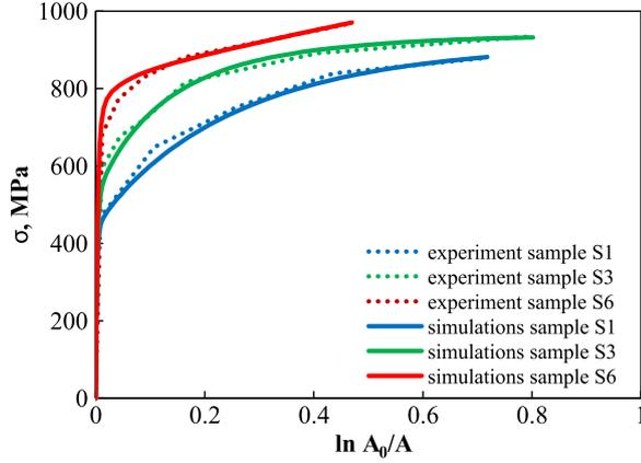
**Fig. 10.** Tensile stress-strain curves: experimental and numerical simulations results.
