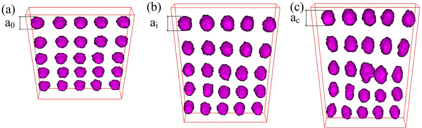
**Fig. 5.** Tomographic reconstruction of a titanium sample containing one array of laser drilled holes. The example is for the S5 sample, that has been tested in-situ and the tomograms correspond to the following true strains (a) 0.00, (b) 0.16, (c) 0.30. The tensile direction is vertical. Initial void diameter  $a_0$  is 35  $\mu\text{m}$ .
