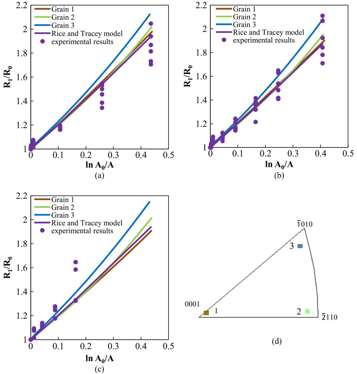
**Fig. 12.** Experimental and simulation results of void growth in three samples: (a) S1, (b) S3 and (c) S6. (d) The inverse pole Fig. shows the three different grain orientations used in the simulations.
