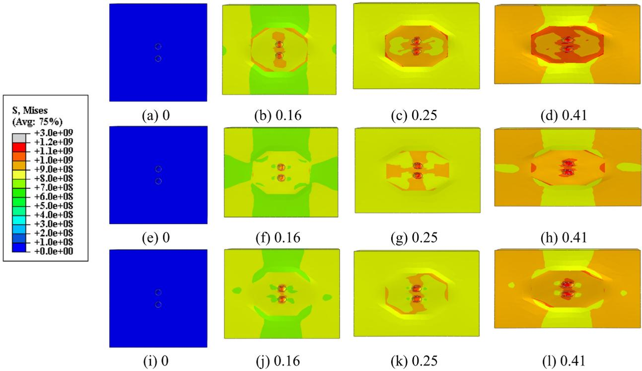
**Fig. 15.** Visualization of void growth for two voids interspaced at 2d for sample S3 in grains with different orientation at different true strains: (a)-(d) Grain 1, (e)-(h) Grain 2, (i)-(l) Grain 3. Tensile direction is horizontal.
