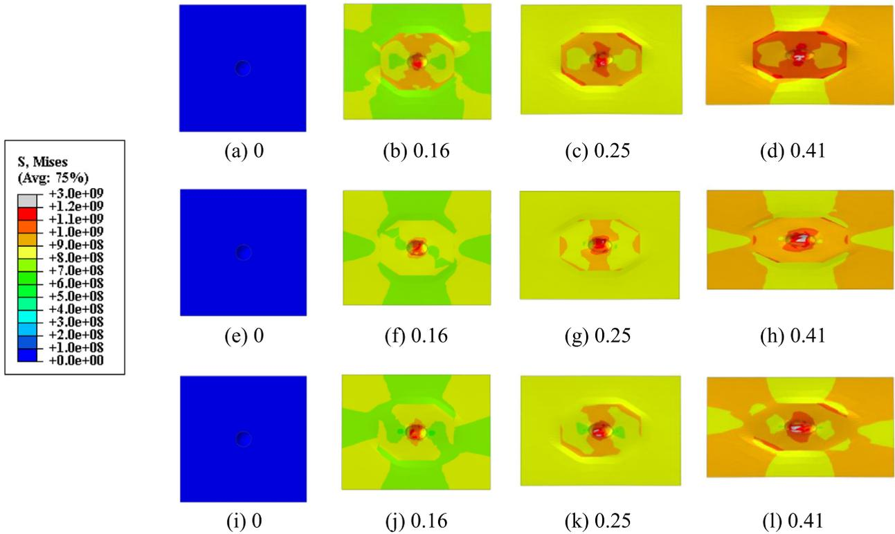
**Fig. 13.** Visualization of void growth for sample S3 in grains with different orientation at different true strains: (a)-(d) Grain 1, (e)-(h) Grain 2, (i)-(l) Grain 3. Tensile direction is horizontal.
