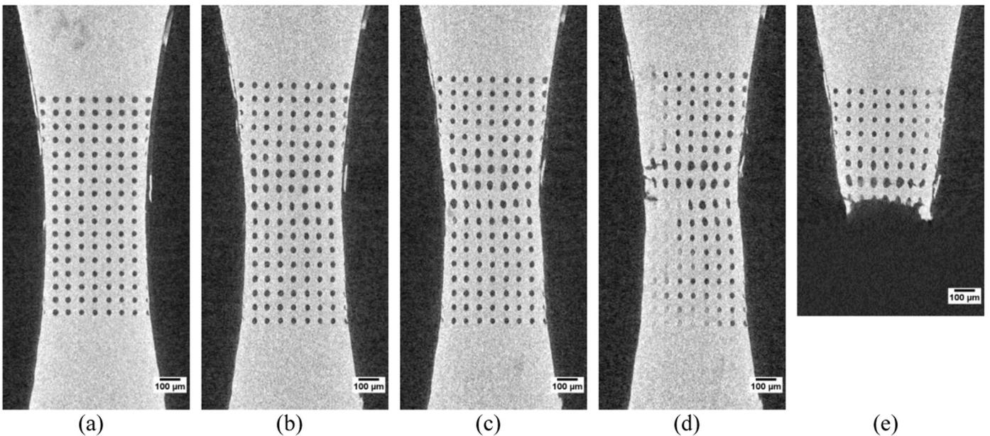
**Fig. 6.** Sequence of tomographic reconstructions showing deformation for a titanium sample (S5) with a rectangular array of voids oriented at  $0^\circ$  with respect to the tensile axis at the following true strains: (a) 0, (b) 0.15, (c) 0.21, (d) 0.32 and (e) at fracture. Tensile axis is vertical.
