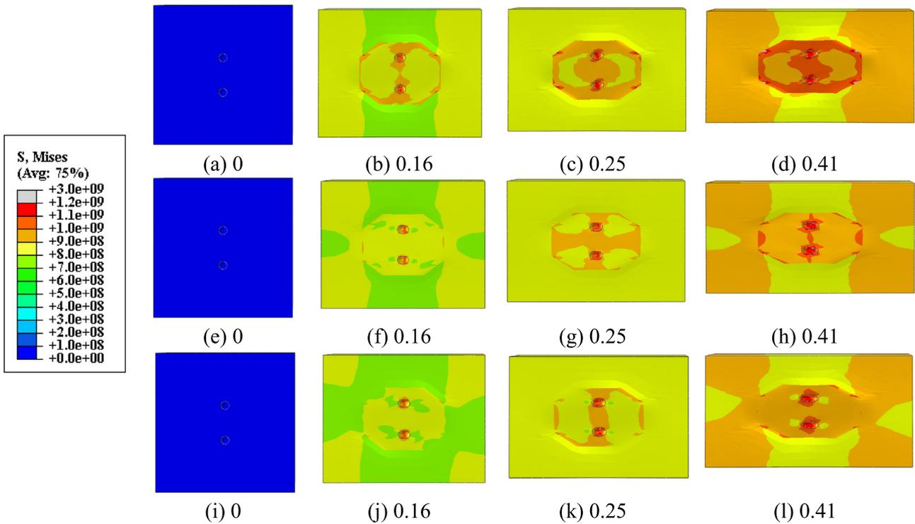
**Fig. 16.** Visualization of void growth for two voids interspaced at 4d for sample S3 in grains with different orientation at different true strains: (a)-(d) Grain 1, (e)-(h) Grain 2, (i)-(l) Grain 3. Tensile direction is horizontal.
