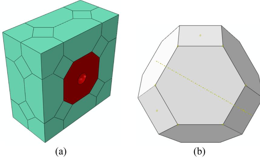
**Fig. 11.** (a) 3D model. Half of the model is shown. Red color indicates crystal plasticity, green color indicates macroscopic properties of titanium; (b) tetrakaidecahedron used to construct the 3D model. (For interpretation of the references to color in this figure legend, the reader is referred to the web version of this article.)
