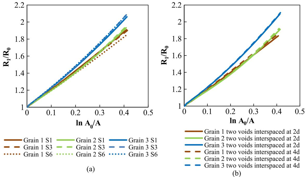
**Fig. 14.** (a) Comparison of void growth simulation results between different samples S1, S3 and S6. (b) Comparison of void growth simulation results for sample S3 for two voids at different interspacings.
