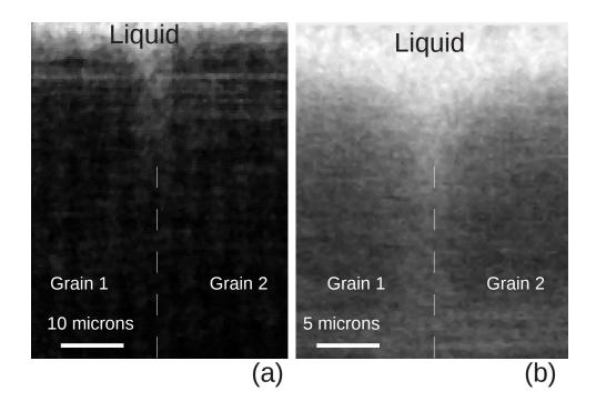
FIG. 6. Projected view of the mobility in a  $\Sigma 5$  (100) (a) and in a  $\Sigma 17$  (100) grain boundary (b). Grooves can be observed at the solid/liquid interface grain boundary tripple line.
