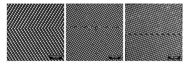
FIG. 2. Confocal images of the templates:  $\Sigma 3(110)$  (left),  $\Sigma 17(100)$  (middle) and  $\Sigma 5(100)$  (right).
