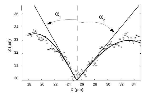
FIG. 10. Fitting of the experimental groove profile.
