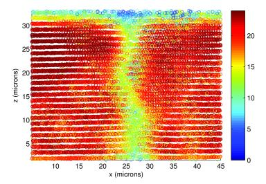
FIG. 3. Projection of the order parameter of all particles in the  $\Sigma 5$  (100) bicrystal. The grain boundary is perpendicular to the plane of the figure and the template is at the bottom. The color bar indicates the order parameter (0–24).
