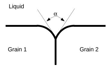
FIG. 1. Definition of the geometry of the groove at the grain boundary – liquid triple junction.
