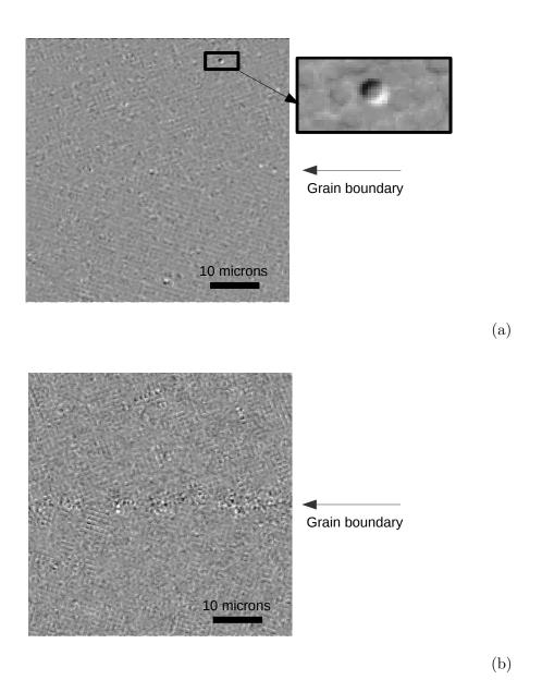
FIG. 5. Difference between two consecutive confocal microscopy images of the same location taken two minutes apart. (a) Slice close to the template at the bottom of the sample and (b) Slice close to the liquid/solid interface. The grain boundary is horizontal in the middle of the images. Some particles have moved, leading to characteristic black and white patterns like the one shown as a zoomed inset in Fig. (a).
