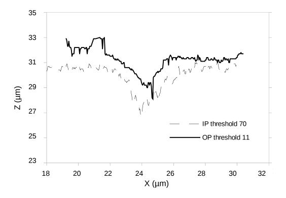
FIG. 9. Comparison of the two best thresholds using the order parameter (OP) and the image processing (IP) procedures.
