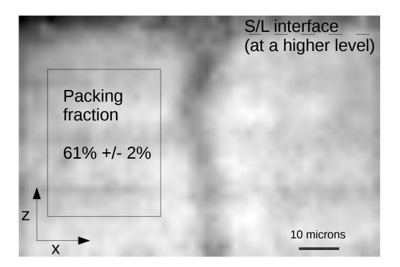
FIG. 12. Average value of the density in the plane perpendicular to the grain boundary (lower densities for darker gray levels). Note that the density is smaller at the grain boundary, at all heights Z.
