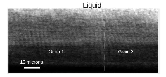
FIG. 7. Projected view of the mobility in a  $\Sigma 3$  (110) grain boundaru. No groove can be observed. of the boundary, defines the profile of the groove.
