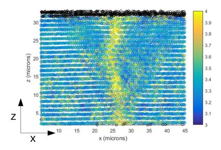
FIG. 13. Average Voronoi volumes of the particles the  $\Sigma 5(100)$  boundary projected onto the x-z plane.
