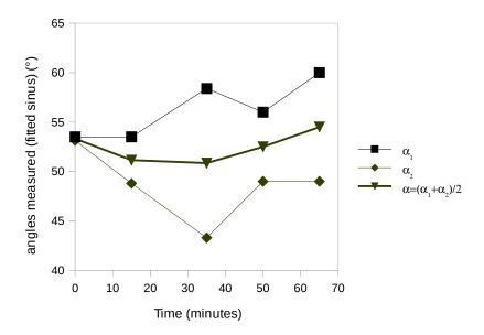
FIG. 11. Time dependence of the two contributions,  $\alpha_1$  and  $\alpha_2$ , to the groove angle  $\alpha$  of the  $\Sigma 5(100)$  boundary. The contributions fluctuate more than the total angle.
