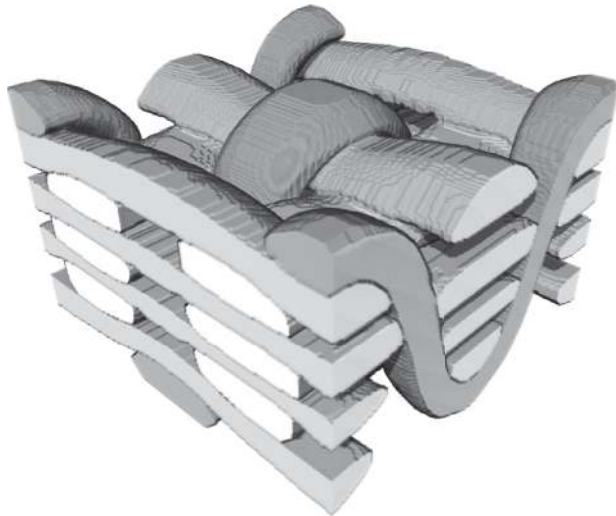
FIGURE 3. 3D orthogonal non-crimp segmented volume.
