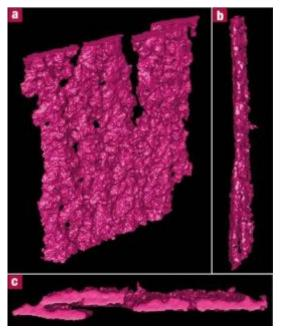
Figure 11: Three-dimensional representation of an isolated lamellar crystal, 1.3 microns particles. Perspective (a), side (b) and top view (c). Crystal height represented: 360 microns. The surface of the crystal is not faceted.
