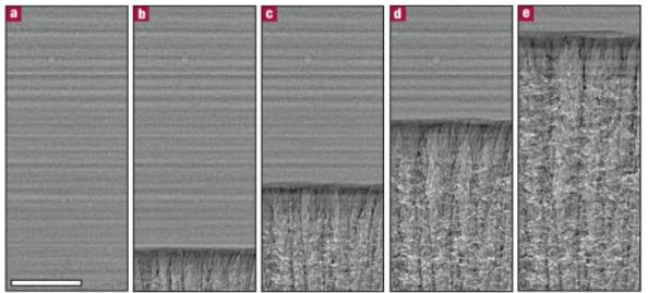
Figure 7: Solidification sequence in the steady state, high resolution radiography, 0.4 microns particles. Time picture was taken:  $a=t_0$ ,  $b=t_0+4s$ ,  $c=t_0+9.7s$ ,  $d=t_0+16s$ ,  $e=t_0+24.7s$ . Scale bar: 150 microns.
