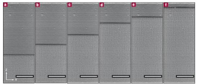
Figure 1: Solidification sequence in the steady state, radiography, 1.3 microns particles. Time picture was taken at:  $a=t_0$ ,  $b=t_0+6s$ ,  $c=t_0+13.7s$ ,  $d=t_0+22.3s$ ,  $e=t_0+27.3s$ ,  $f=t_0+34.7s$ . Scale bar: 500 microns.
