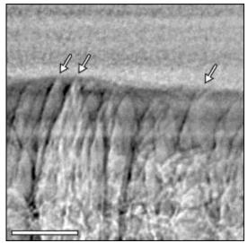
Figure 8: Detail of the solidification sequence in the steady state (Figure 7), high resolution radiography, 0.4 microns particles. Details of the dendrites tip. No visible concentration of particles ahead of the dendrites tip is observed. Interface velocity: 20 microns/s. Scale bar: 50 microns. Arrows indicate the dendrites tip. The solidification front is moving vertically, bottom to top.
