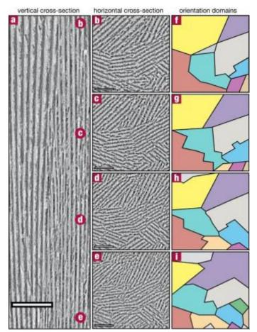
Figure 3: Reconstruction from tomography acquisition, 1.3 microns particles. Vertical (a) and horizontal (b-f) cross-sections of the frozen arrangement. The corresponding orientation domains, corresponding to domains of long range order of the crystals alignment, are given in (f)-(g). Scale bars : a : 300 microns, b-e : 150 microns.
