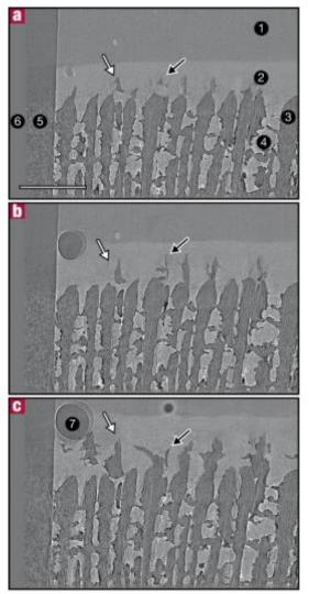
Figure 14: Solidification sequence, in situ tomography, 0.4 microns particles. Evidences of constitutional supercooling. The solidification front is moving vertically, bottom to top. Scale bar: 500 microns. Legend: 1: unfrozen suspension, 2: concentrated particles ahead of the interface, 3: ice crystals, 4: concentrated particles surrounded by ice 5: polymer mold, 6: outside background, 7: bubble. Approximate time: a: to, b: to+30s, c: to+60s.
