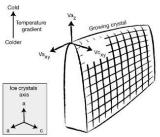
Figure 13: Growth velocities and crystal orientation. Ice, under these conditions of temperature and pressure, is hexagonal, with strong anisotropies of interface kinetics between the a and c axis, resulting in platelets-like crystals.
