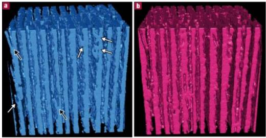
Figure 4: Three-dimensional representation of a block of lamellar ice crystals (left) and corresponding particles entrapped (right). Block dimension: 360x360x360 microns<sup>3</sup>, 1.3 microns particles. White arrows indicate the protruding dendrites, which can eventually turns into lamellar crystals, black arrows indicate twin dendrites, probably resulting from tip splitting.
