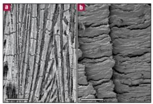
Figure 15: Evidence of local instabilities in the frozen structure (a), leading to large crack-like defects in the final structure (b). Scale bars: 200 microns. a: tomography picture, b: SEM picture after sublimation and sintering.
