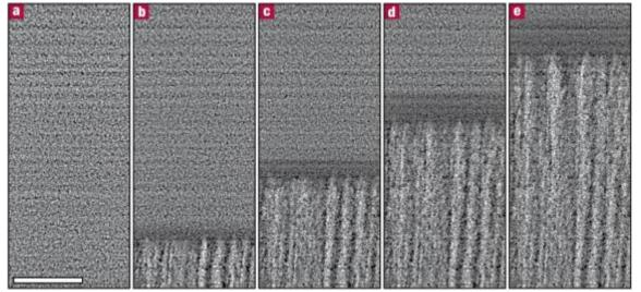
Figure 9: Solidification sequence in the steady state, high resolution, 3.4 microns particles. Time picture was taken:  $a=t_0$ ,  $b=t_0+4s$ ,  $c=t_0+9.7s$ ,  $d=t_0+16s$ ,  $e=t_0+24.7s$ . Scale bar: 150 microns.
