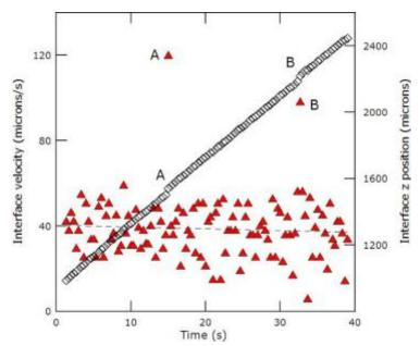
Figure 2: Interface location ( $\Diamond$ ) and velocity ( $\blacktriangle$ , dashed line: linear fit) vs. time, steady state, 1.3 microns particles. The average velocity of the interface is 39 microns/s. The z=0 position corresponds to the position of the interface in Fig. 1a (time t<sub>0</sub>). The velocities peaks noted A and B are significant, but will be discussed in a separate paper.
