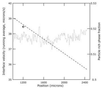
Figure 5: Interface velocity (fit, dashed line) and particle fraction (continuous line) vs. position of the interface, steady state, 1.3 microns particles. The z=0 position corresponds to the bottom of the picture in Fig. 1a. No significant variations of the particles fraction are observed.
