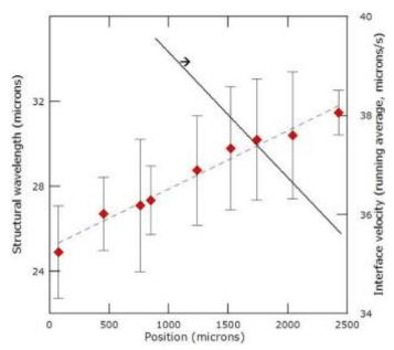
Fig. 6: Structural wavelength ( $\Diamond$ ) and interface velocity (fit)( $\triangle$ ) vs. position, as measured on reconstructed cross-sections. 1.3 microns particles.
