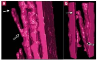
Figure 12: Growth termination of dendrites, three-dimensional representation. Black arrows indicate the origin of the dendrites and white arrows their termination. The dendrites can either stop in between the crystals (a), or reach the next adjacent crystal (b).
