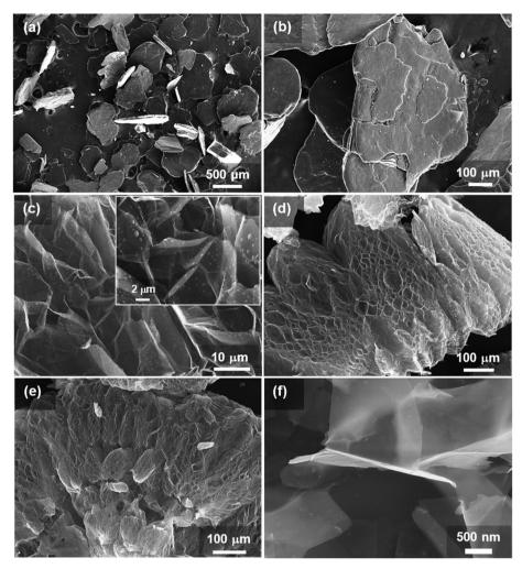
**Fig. 1.** FEC-SEM micrographs of (a), (b) as received expandable graphite flakes, (c) EG powder prepared by abrupt heating of expandable graphite at 900 °C for 10 s. Inset reveals the bubbles on the layers due to incomplete gas release, (d) EG powder prepared at 900 °C for 1 min, (e) EG powder prepared at 900 °C for 2 min and (f) exfoliated material obtained by tip sonication of EG in IPA for 90 min followed by centrifugation (EG-IPA-90 min-TS).
