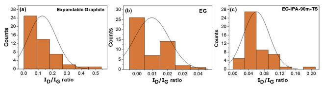
Fig. 7. Statistical histogram of the  $\frac{l_D}{l_C}$  ratios derived from 50 Raman spectra recorded at different locations. (a) Expandable graphite, (b) EG, and (c) EG-IPA-90 min-TS sample. The distribution curves indicate the mean of the data.
