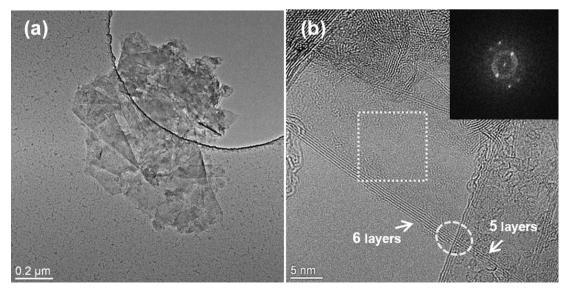
Fig. 12. (a) TEM image of exfoliated sample deposited from PA-IPA-90 m dispersion. (b) HRTEM micrograph of few-layer graphene sheets with an amorphous coating on their surface deposited from the PA-IPA-90 m dispersion. Inset of (b) shows the FFT image of the area indicated by a dashed rectangle.
