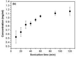
**Fig. 2.** Concentration of graphene-based material remaining after centrifugation at 500 rpm for 45 min as a function of sonication time (a) for the IPA- and NMP-based dispersions prepared by bath sonication of SEFG and PA powders and a following centrifugation at 500 rpm for 45 min (the results for the SEFG-IPA dispersions which were centrifuged at 900 rpm for 45 min and the EG-IPA dispersions were also shown in the plot, for comparison), and (b) for the SEFG-IPA dispersions.
