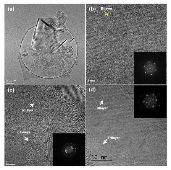
**Fig. 11.** (a) TEM image of few-layer (<5 layers) graphene sheets achieved after sonication of SEFG in IPA for 90 min followed by centrifugation (SEFG-IPA-90 min sample). HRTEM images of SEFG-IPA-90 m sample showing (b) a bilayer graphene, (c) few-layer (<5 layers) graphene sheets and graphite flakes, and (d) SEFG-IPA-90 m sample annealed at 2600 °C in Ar atmosphere for 4 h revealing bi-layer and three-layer graphene sheets. Insets show the FFTs of the corresponding HRTEM micrographs.
