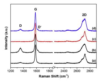
**Fig. 5.** Representative Raman spectra (normalized to the G-band) of (a), (b) expandable graphite ((a) and (b) show the Raman spectra recorded at different locations of the laser spot over the thin film), (c) expanded graphite (EG), and of (d) exfoliated (EG-IPA-90 min-TS) sample.
