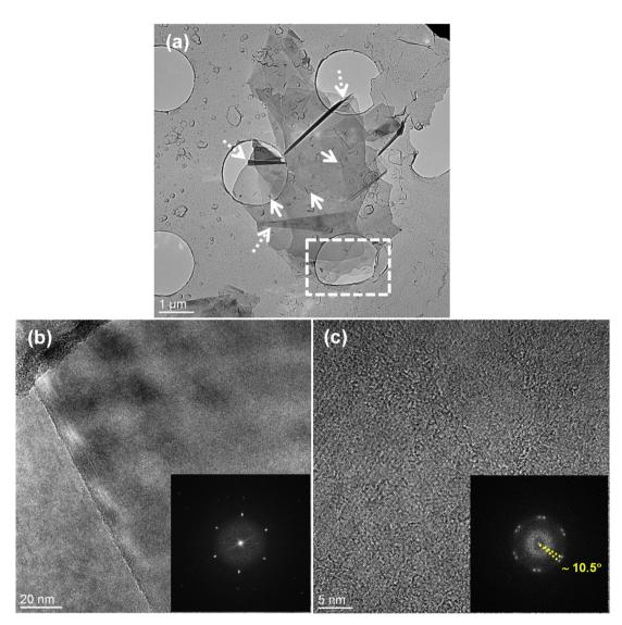
**Fig. 10.** (a) TEM image of graphene flakes deposited from EG-IPA-90 min-TS dispersion. Dashed arrows show the folded regions, solid arrows show the wrinkles and dashed box indicates the graphene layers on top of each other. (b) A HRTEM image of the EG-IPA-90 min sample. Insets show FFT of the corresponding HRTEM image. (c) HRTEM image of a turbostratic graphene showing an amorphous layer covering the surface. It's FFT (inset) indicates a rotation angle of 10.5°.
