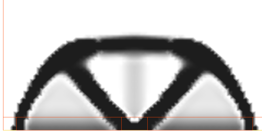
Figure 4: Numeric results for case B : Optimal density
